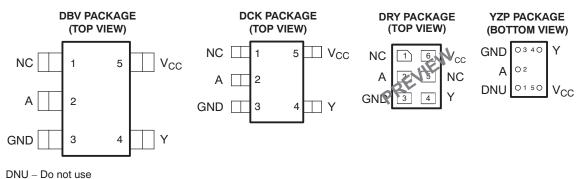
NC – No internal connection See mechanical drawings for dimensions.
